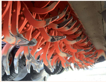
Hooks mounted irregularly
